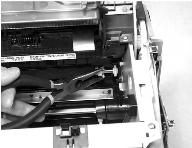
Figure 5-22 Remove the transfer roller (3 of 3)
